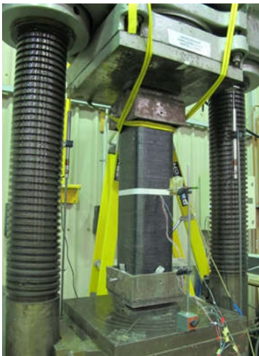
Figure 10. Strengthening rectangular columns with hoop FRP sheets
