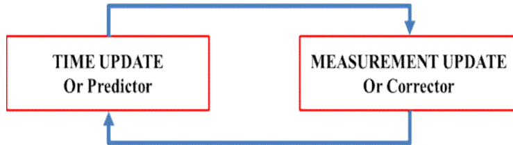
Figure 2. Continuous cycle of Kalman filter
