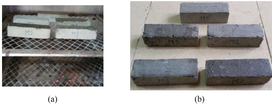
Figure 3. (a) Heat resistance test; (b) samples after heat resistance test
