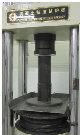
Figure 4. Compression test of concrete cylinder
